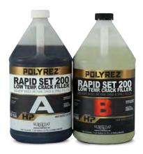
Rapid Set 200 is an extremely fast setting, high strength, ultra low viscosity concrete repair material designed specifically for use in cold weather environments. This two-part, hybrid urethane system is designed for rapidly rebuilding deeply spalled or damaged concrete surfaces, broken control joints and rapidly repairing damaged concrete, especially in cold conditions. Rapid Set 200 can accept heavy loads and be ground smooth in 10 - 15 minutes in temperatures between 20° - 40° F.
